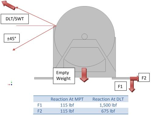
Forces are maximum forces per bolt, at SWT & DLT, for a 4 bolt hold down pattern (Rows spaced at 48"). Analysis is good for a vertical fleet angle of  $\pm 45^{\circ}$  and a horizontal fleet angle of  $\pm 8^{\circ}$ .
